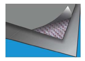
A Pure Graphite sheet with tanged stainless steel reinforcement for improved blow out resistance and ease of handling. UKL GPS is mechanically bonded with an excellent Chemical resistance & Thermal properties. Widely used in Petrochemical, Oil & Gas, Steel, Chemical and Automobile industries. Application includes high pressure, high temperature Steam, Exhaust and Speciality chemicals.
